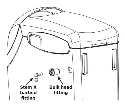
Make sure the pipe us not run higher than the fitting on the cabinet and is kink-free.
