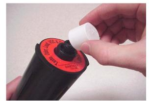
Figure 3. Filter Cartridge Cap Removal
